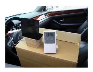
Without FUMIN COATING After IR light irradiation :  $31.5^{\circ}$ C
